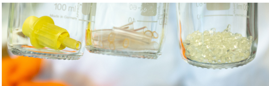
GARD™skin Medical Device can be used for testing of skin sensitization with extraction vehicles according to ISO 10993-12:2012.
