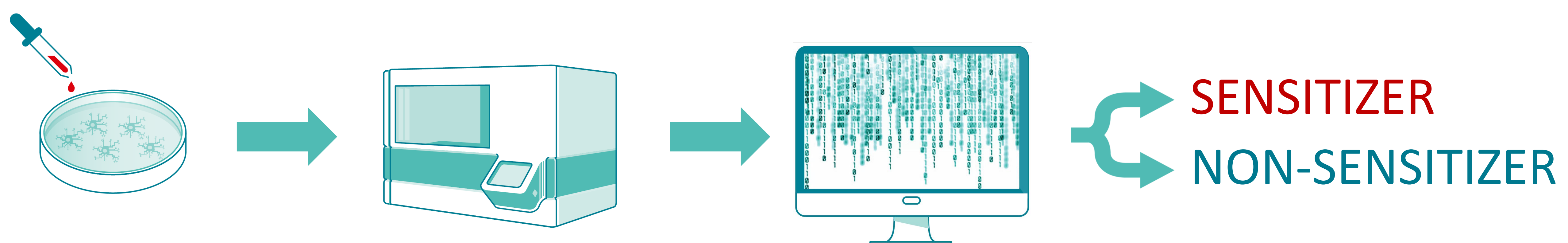
Figure 2. The GARD test principle. The cultivated cells are exposed to test substances for 24 h. mRNA is isolated and hybridized to reporter probes. After automated measurement and data acquisition, the transcription levels of the predictive signature (200 genes) are analyzed, and each sample is given a decision value as either sensitizer or non-sensitizer, based on SVM classifications.
